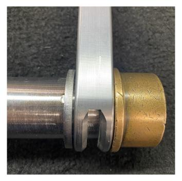
Now place (3) tack welds, welding the spacer rings to the ARB main tube.
