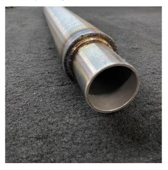
The Anti-Roll Bar arms must be tig welded to the inner & outer tube. If other methods are used, your welds may not clear the chamfer on the bronze bushings. This could cause the Anti-Roll Bar to not be able to freely travel through its necessary range of motion.
