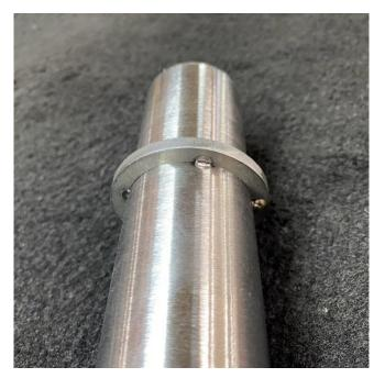
Then fit the outer tube over the spacer rings, THIS WILL BE TIGHT. Place (1) tack weld on each spacer ring to the outer ARB tube.
