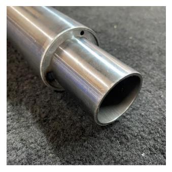
Now weld the spacer rings to both the inner & outer ARB tubes.
