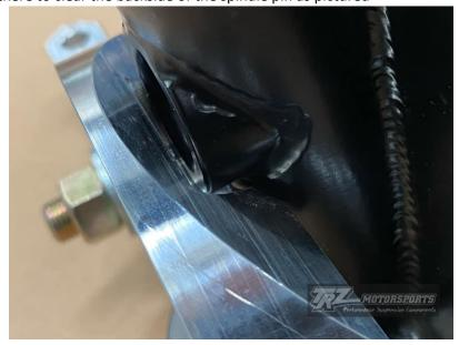
Spindle spacers go between the steering arm & the spindle itself
