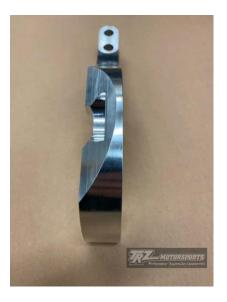
The notch on the rear of the steering arm should be facing the inside of the spindle
