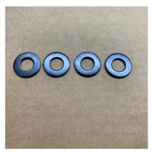
Some ball joints include washers to account for variations in spindle taper
