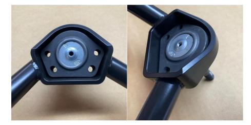
You will align the ball joint in the cup by using the top two bolts / holes
