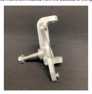
You may use loctite if you'd like. The caliper mounting bracket hardware will pull the inserts through the spindle upon tightening them.
