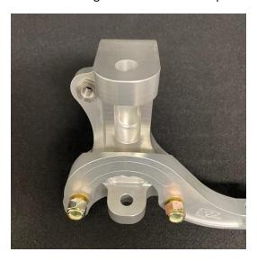
Supplied inserts are installed from the backside of the spindle.
