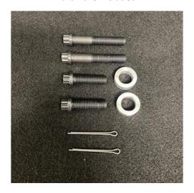
Use a dab of red Loctite on steering arm hardware & torque to 30 ft lbs
