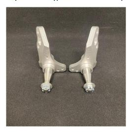
Spindles are not the same & need to be installed in the correct orientation
